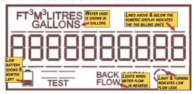
Low-Flow Indicator — The low flow indicator illuminates and turns if water is flowing through the meter.
