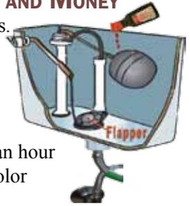
**1st** - put a couple of drops of food coloring in the tank and leave it for an hour or two. If the bowl water changes color the flapper needs to be replaced.
